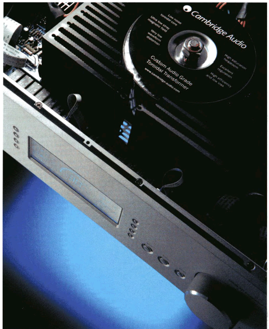
Solid engineering: the massive transformer in the Azur 840A amplifier
